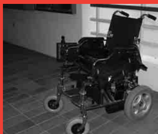
A standard power wheelchair with rear wheel drive allows users to travel faster
